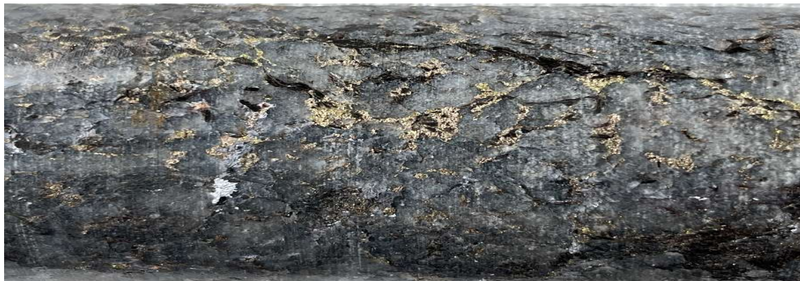
Figure 1. Mineralization in Diamond Drill Hole PIPY25-08 – Interval Assayed 2.65 g/t Au, 36.2 g/t Ag and 2.83% Pb
