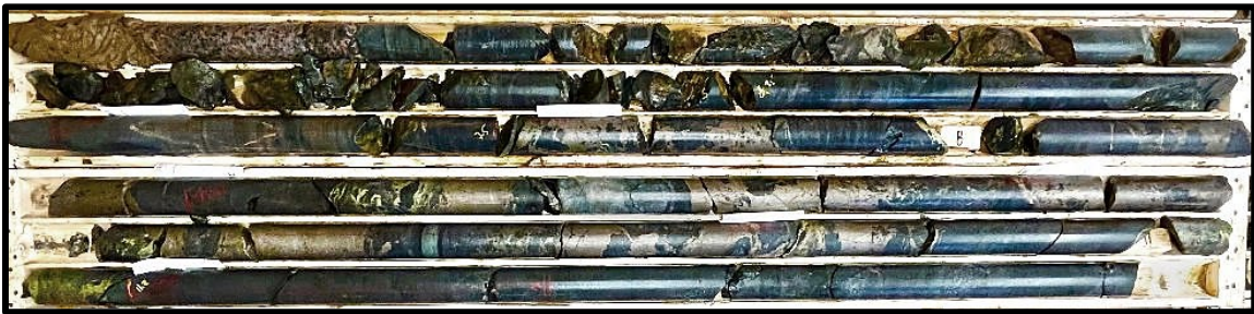
Figure 1. Diamond Drill Hole Wine 24-1A (6.4m-12.5m) New Northern Zone Mineralization (From 7.5m-11.2m – 1.89% NiEq over 3.7m)
