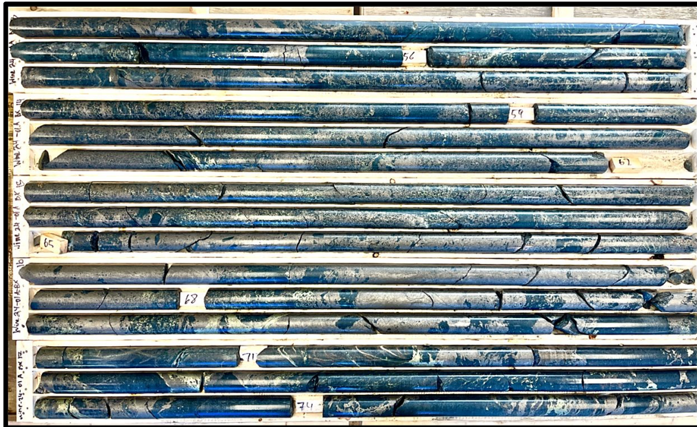
Figure 2. Diamond Drill Hole Wine 24-1A (53.45m-75.1m displayed) Main Zone Mineralization. Displayed section represents 21.65 meters that averages 1.99% NiEq.
